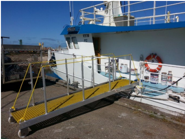
An example of a boarding platform recently built by the owner of a prawn trawler
